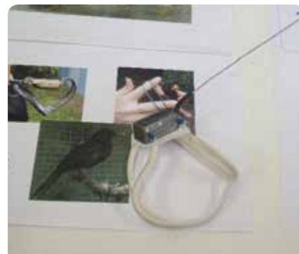
SLAM: Example of a harness with a tag and antenna
