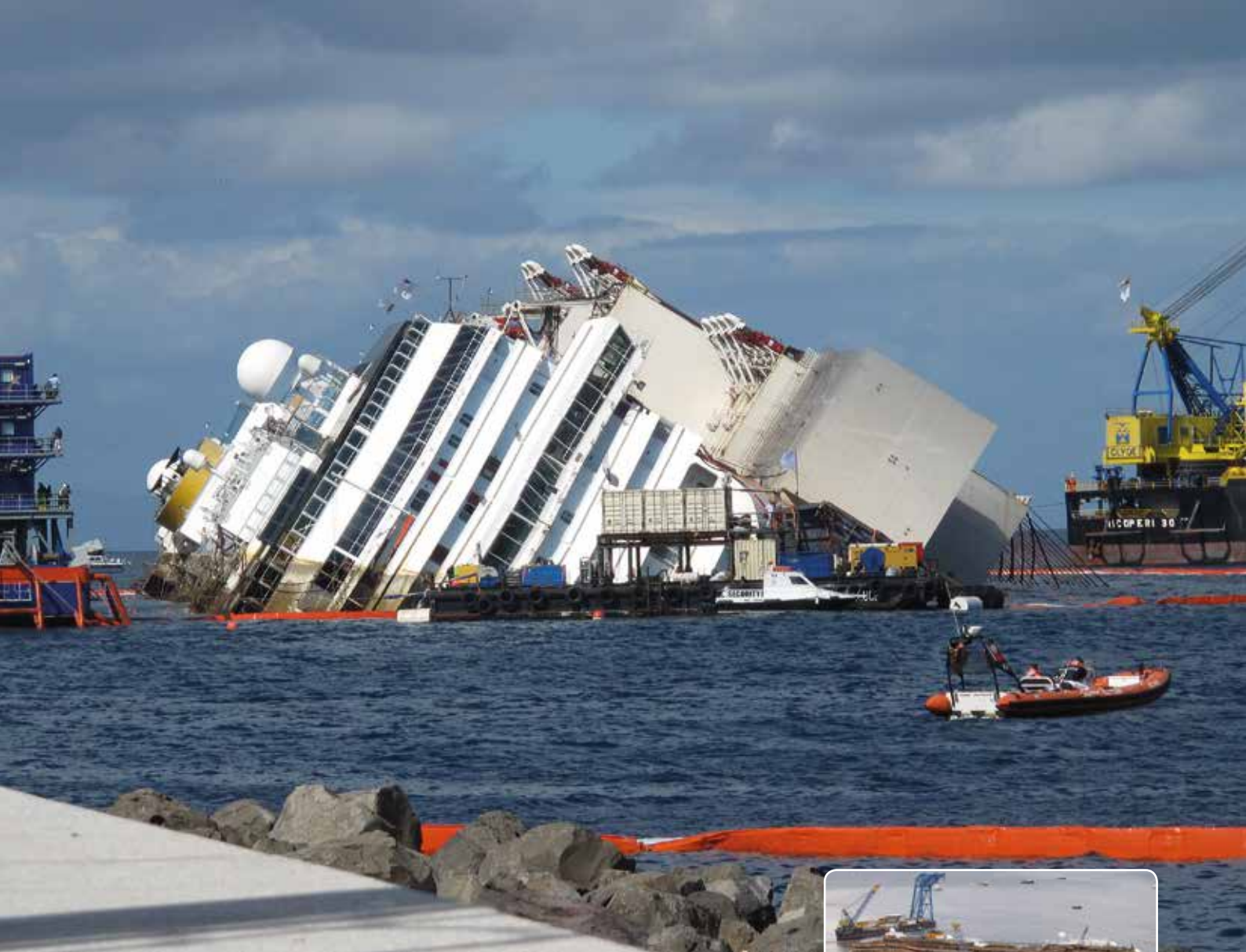
Boom surrounding the COSTA CONCORDIA as the parbuckling operation gets underway
