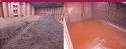
Iron fines before and after liquefaction 2 (Photos courtesy of Brookes Bell)
