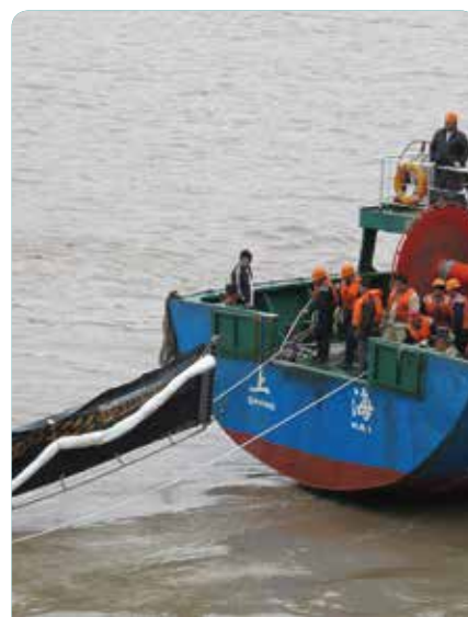
Deployment of boom by a SPRO following a spill from a container ship in the East China Sea
