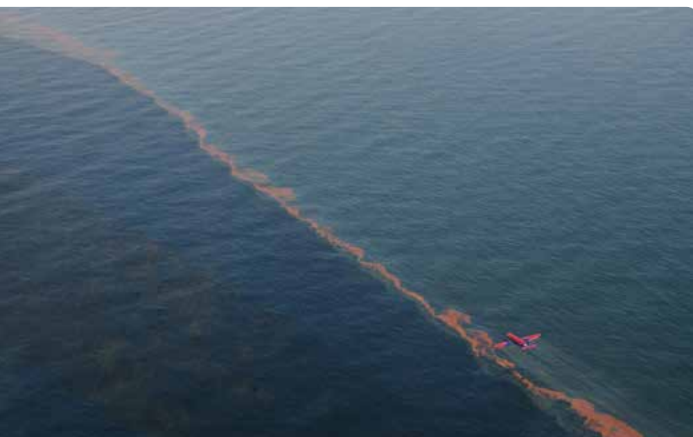
Aerial application of dispersant following the DEEPWATER HORIZON spill (Photo courtesy of Lehmann/USCG)
