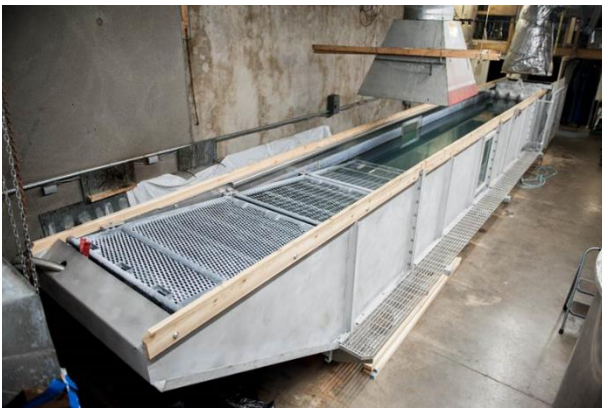
Figure 4-1: SL Ross wind/wave tank
