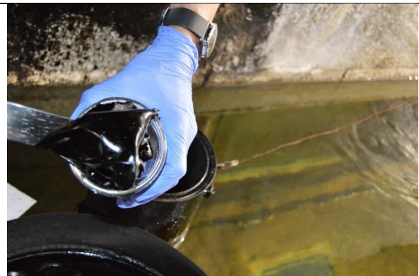
Figure 4-7: Test burn residue recovery from burn ring
