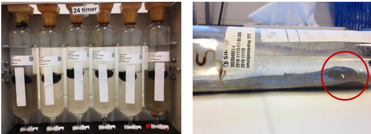
Figure 5-7 Left: Water uptake of 200 and 250 °C+ residues after 24 hours weathering at 2°C. Right: Waxy lump (red circle) formed from the 250°C+ residue of ULSFO Shell 2019 at 13 °C
