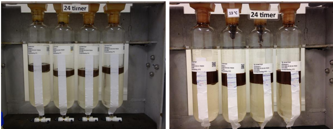
Figure 5-4 The rotating cylinders of water-in-oil emulsion of VLSFO Chevron 2019 after 24 hours of rotation at 2 °C (left) and 13 °C (right)
