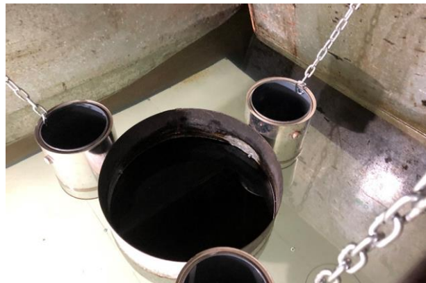
Figure 4-2: 40-cm diameter containment/burn ring
