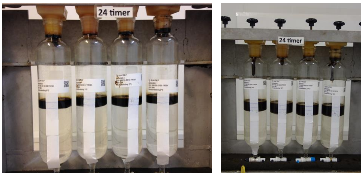
Figure 5-5 The rotating cylinders of water-in-oil emulsion of VLSFO Shell 2019 (fresh oil) after 24 hours of rotation at 2 °C (left) and 13 °C (right)
