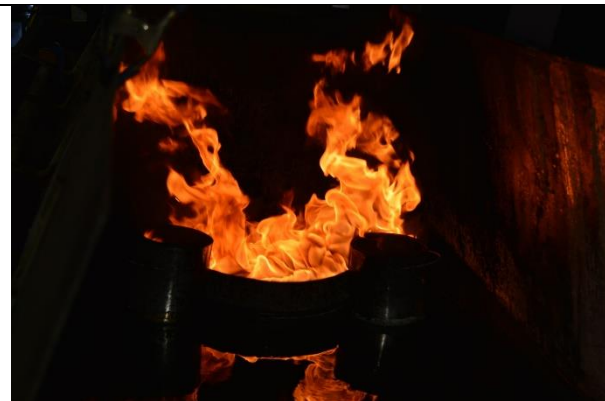
Figure 4-6: Test burn in 40cm burn ring
