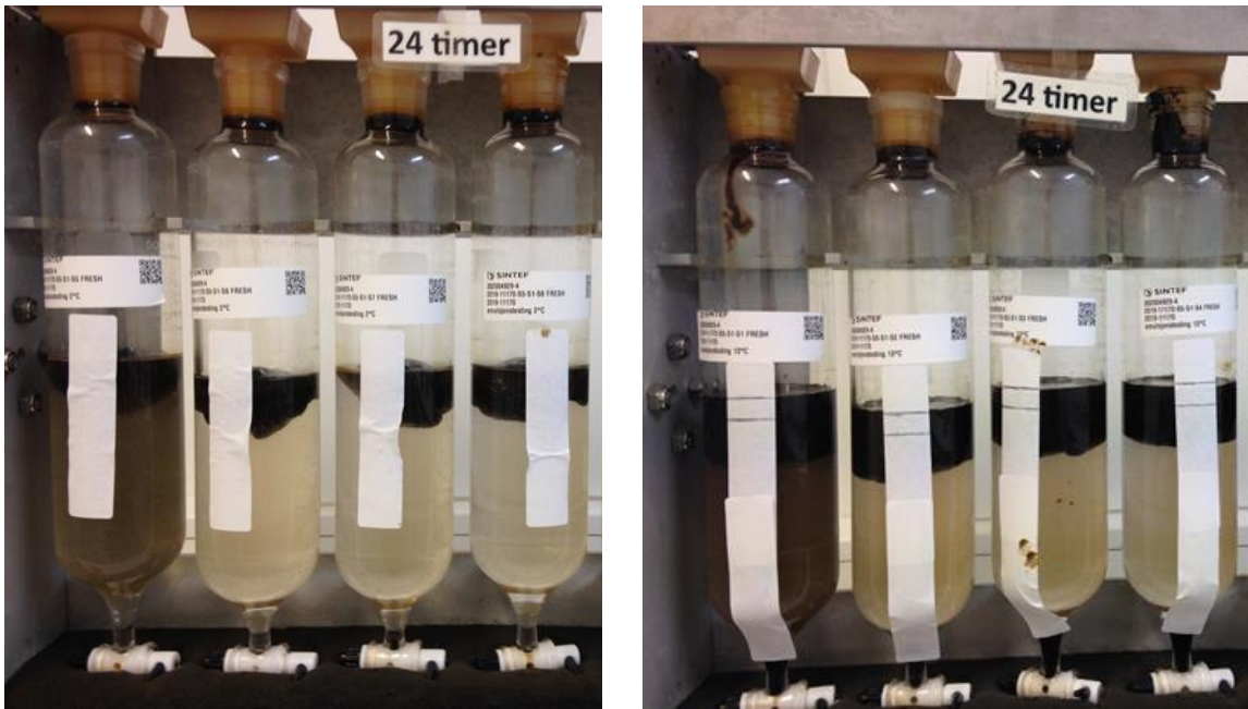
Figure 5-6 The rotating cylinders of water-in-oil emulsion of ULSFO Shell 2019 after 24 hours of rotation at 2 °C (left) and 13 C (right)
