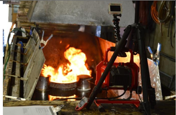
Figure 4-5: Burn conducted between heat shields, under exhaust shroud
