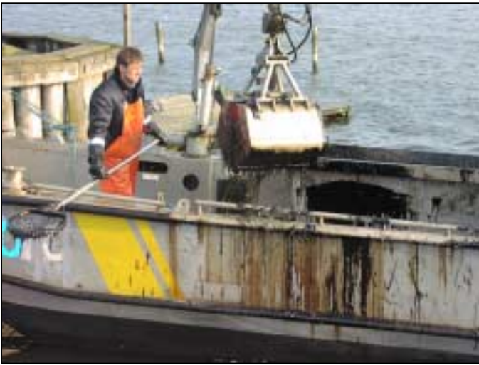
Oil recovery using Danish vessels. The high viscosity of the oil has meant that mechanical grabs rather than skimmers were used.
