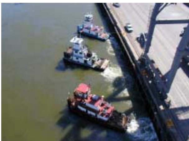
The "Big Flush". Four tugs were used to force oil from beneath the quay
