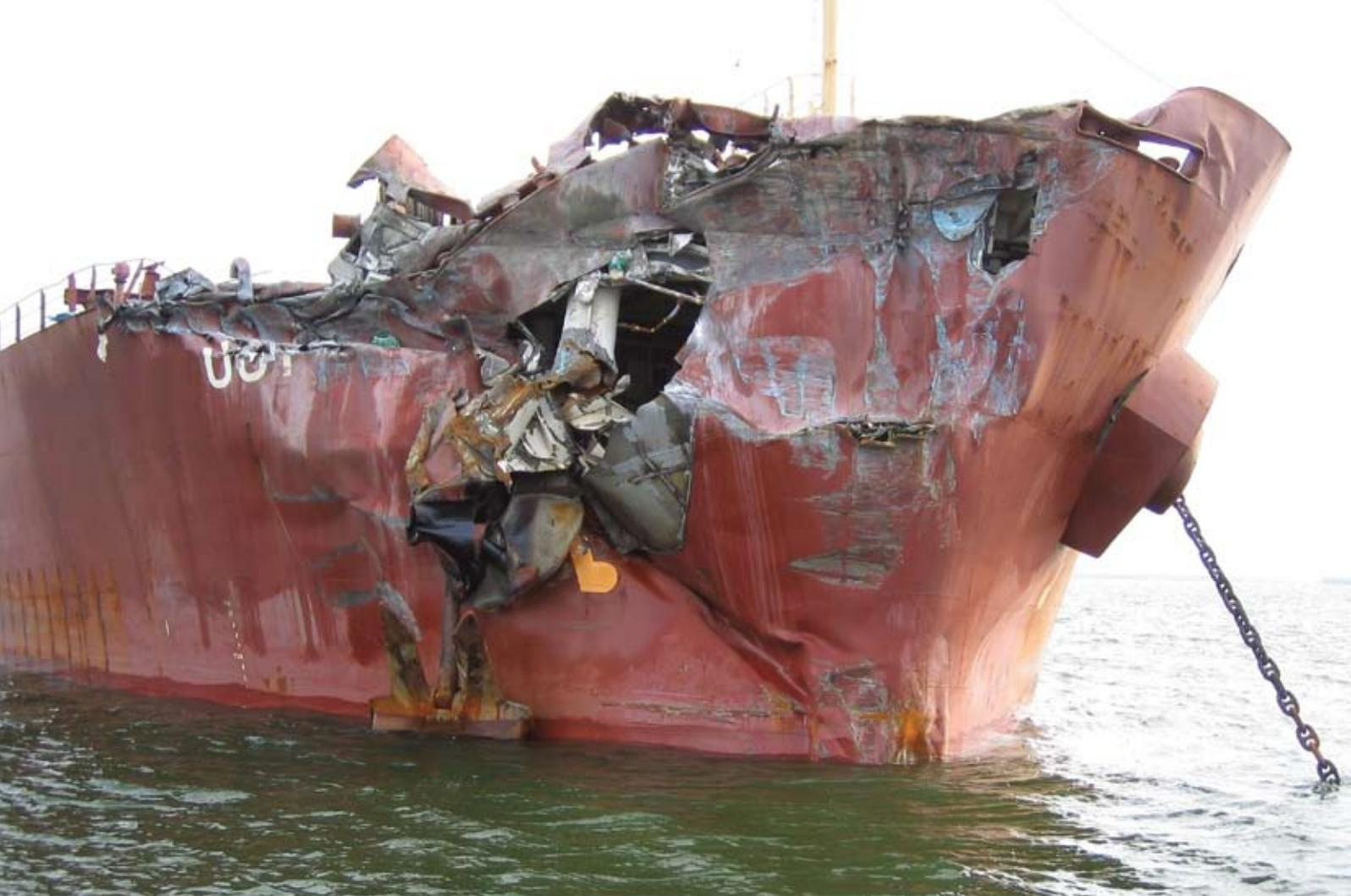
▲ Severe damage sustained in the collision between PEQUOT and MAERSK HOLYHEAD
