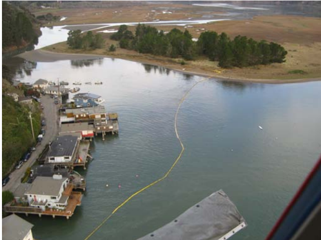
Protective boom in channel
