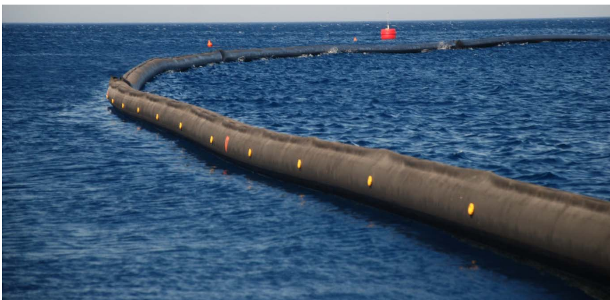
Photo 3: Inflatable boom used in SEA DIAMOND enclosure (July, 2007)
