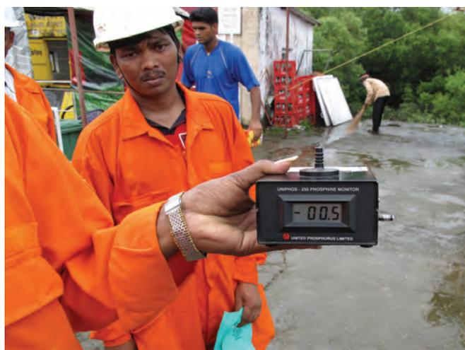
▲ *Figure 14: Demonstration of a hand-held phosphine gas monitor outside a hazardous area.*
