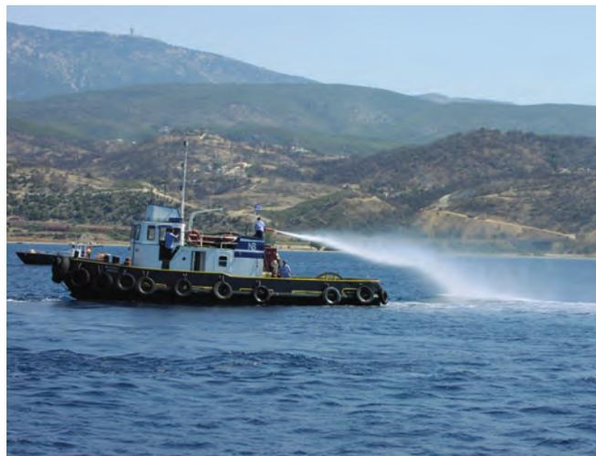
▲ *Figure 8: Application of dispersant using fire monitors on a tug, showing uneven spread of dispersant and the effect of wind.*
