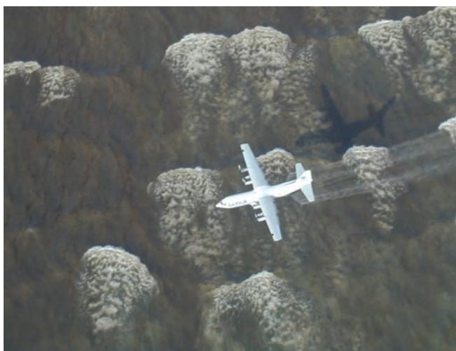
▲ *Figure 10: Application of dispersant from a multi-engine aircraft. Here, application in shallow waters was considered beneficial.*
