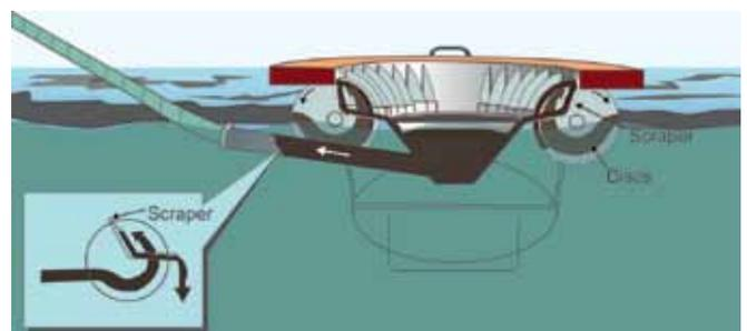
▲ *Figures 2 and 3: Small oleophilic disc skimmer, suitable for oils of medium viscosity. Oil adheres to the rotating discs to be scraped off into a sump for pumping to storage. Requires a suitable pump and hydraulic power supply.*
