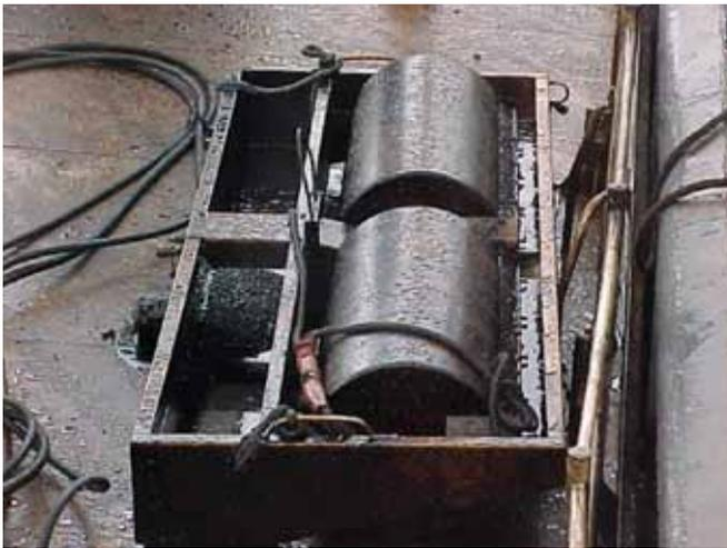
▲ *Figure 4: Oleophilic drum skimmer, suitable for oils of medium viscosity. Operates in a similar manner to a disc skimmer in that oil adheres to the rotating drums to be scraped off into a sump for pumping to storage.*
