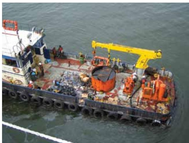
▲ Figure 24: A workboat with limited recovered oil storage on deck.
