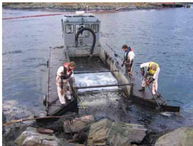
▲ *Figure 34: Self-propelled weir skimmer recovering oil at a sheltered rocky inlet. The shallow draft of the vessel allows work close to shore. Operators assist by moving oil towards the mouth of the weir.*
