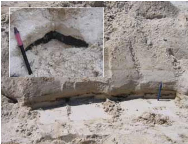
▲ *Figure 12: Layers of oil buried between clean sand by wave action.*
